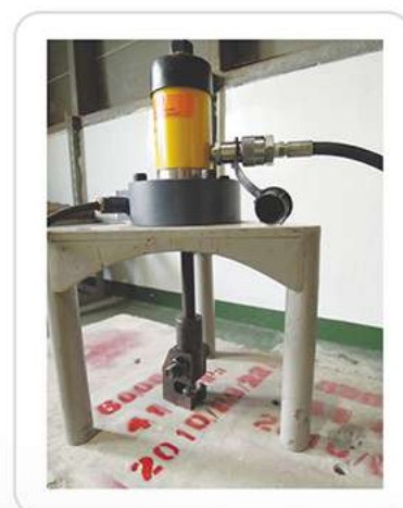
Pull out test
